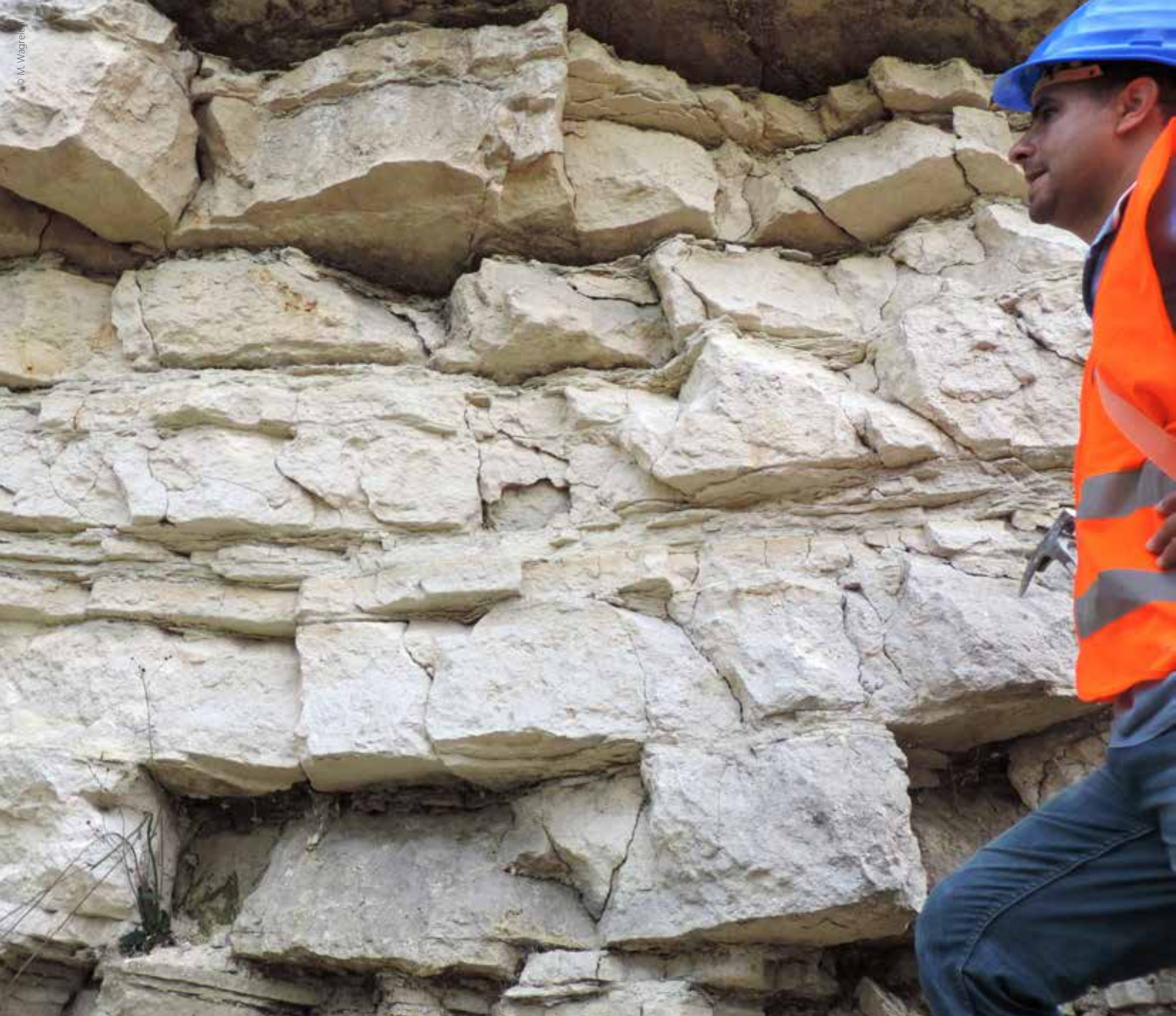
Field work at the so-called Leitha limestone quarry in the south of Vienna, where samples are taken for porosity and permeability measurements
