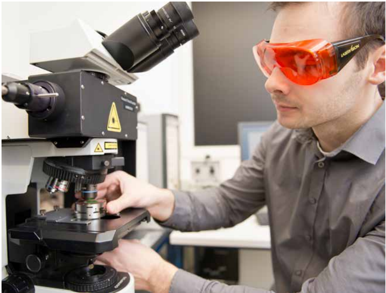
Postdoc Martin Ende adjusts a diamond-anvil cell for an in-situ experiment collecting high-pressure Raman spectra at a Raman microspectrometer.
