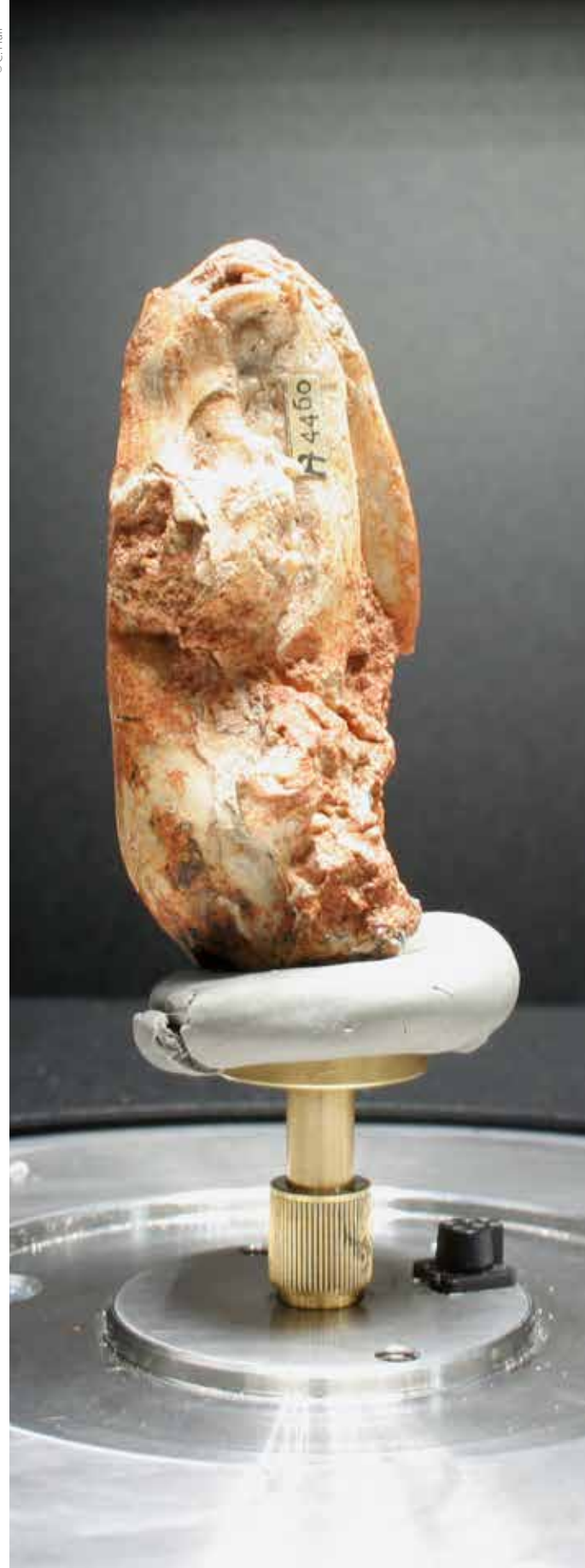
Rare fossil material (e.g. the oldest known cat, Proailurus lemanensis , from Quercy, France) can be investigated non-invasively with high-resolution micro-CT scanning (Bruker/Scyscan 1173).
