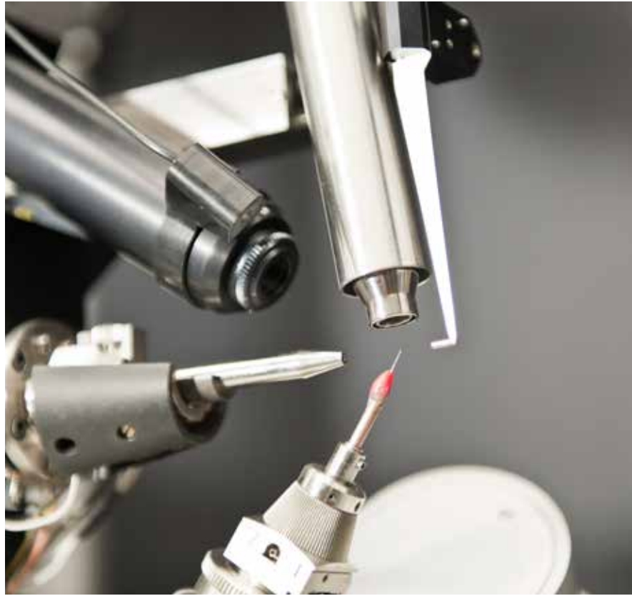
Performing single-crystal X-ray diffraction under low-temperature conditions
