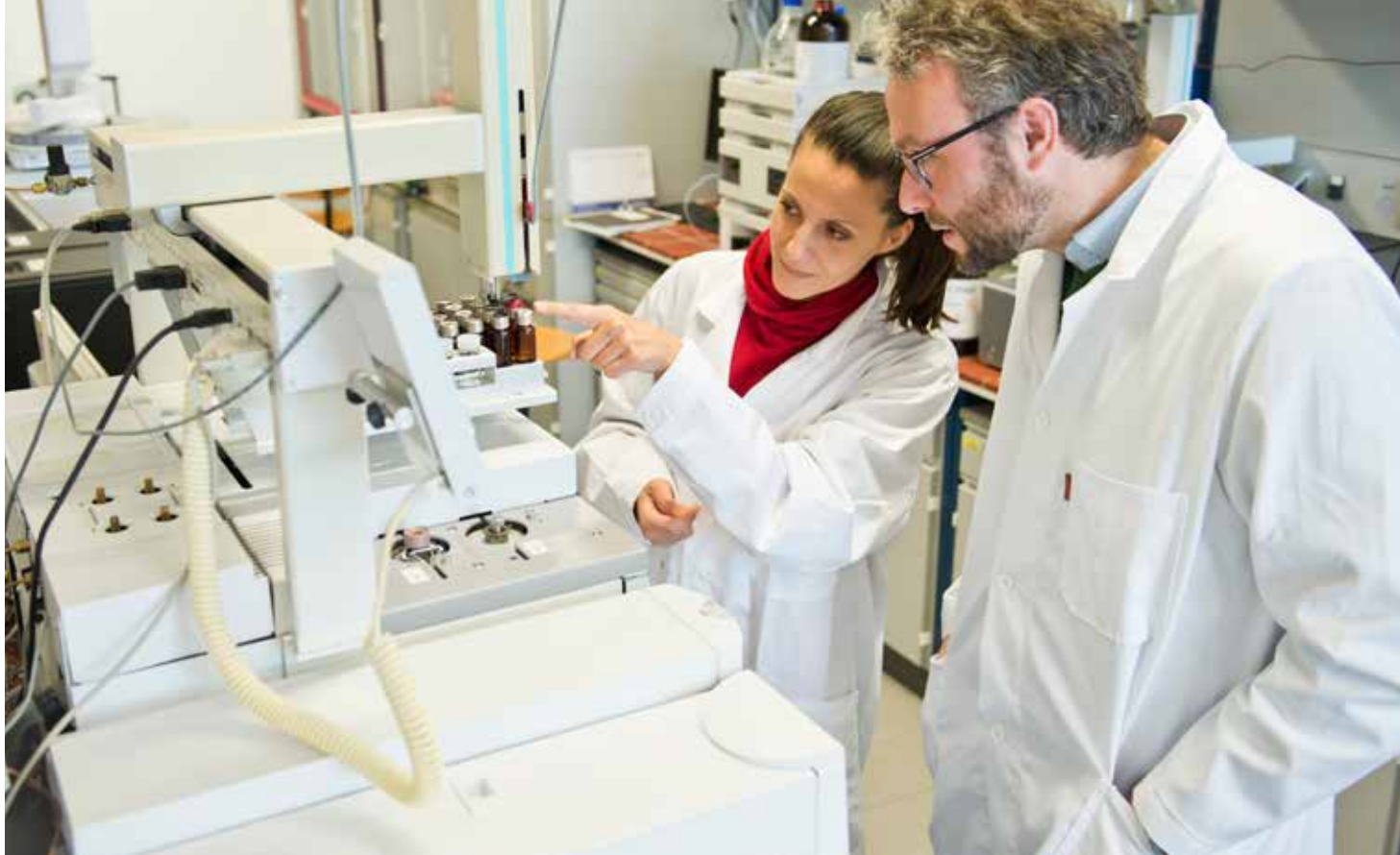
Loading an auto-sampling rack on a gas chromatography/mass spectrometry system to analyse traces of poly-aromatic hydrocarbons (PAH), a widespread organic contaminant in the environment
