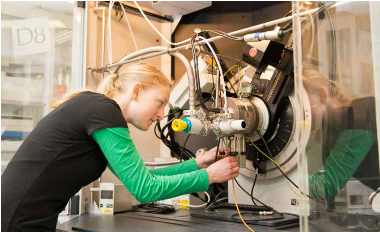
Sigrid Reiter, working on her master's thesis at the Department of Mineralogy and Crystallography, changes the sample in the Paar HTK1200 high-temperature camera, preparing a temperature-resolved XRD measurement under controlled atmospheres of up to 1,200°C.
