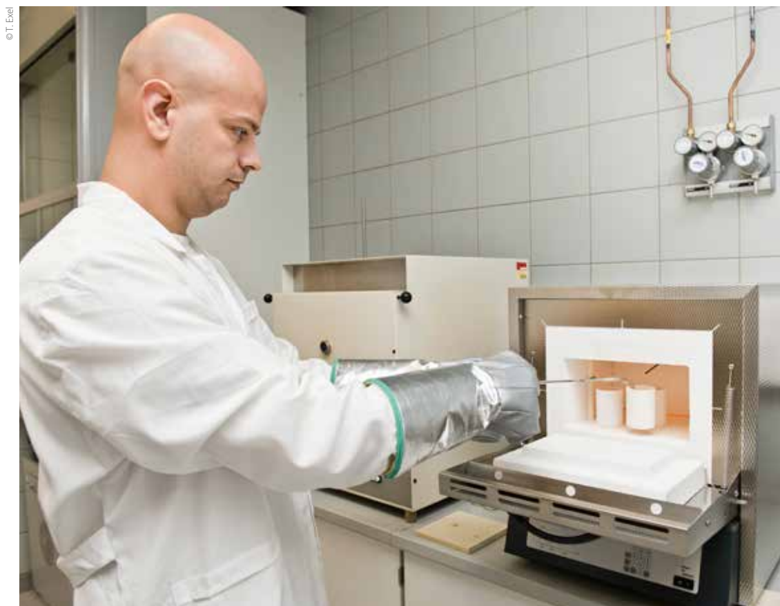
Extraction of aluminium oxide crucible from a high-temperature furnace at 900°C
