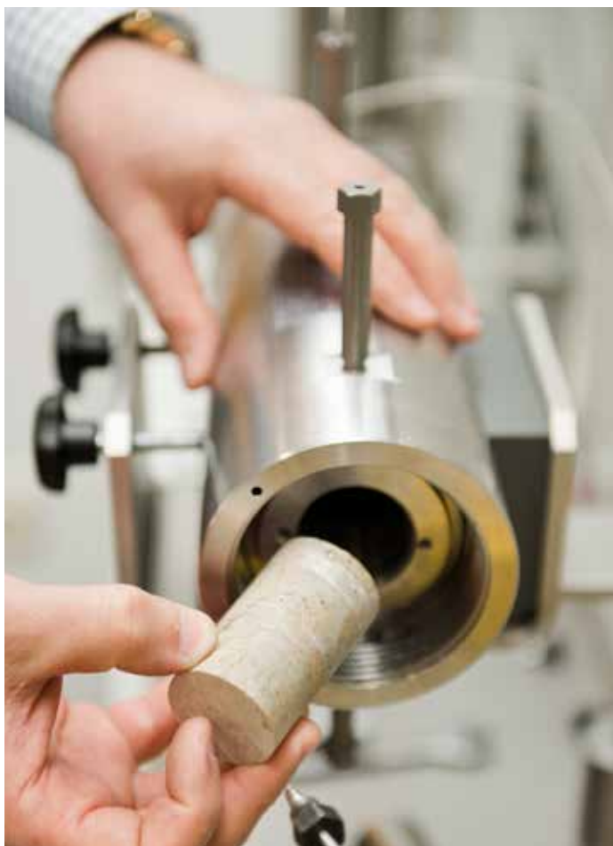
Cut rock sample used for measuring permeability, i.e. the rate of fluids passing the rock
