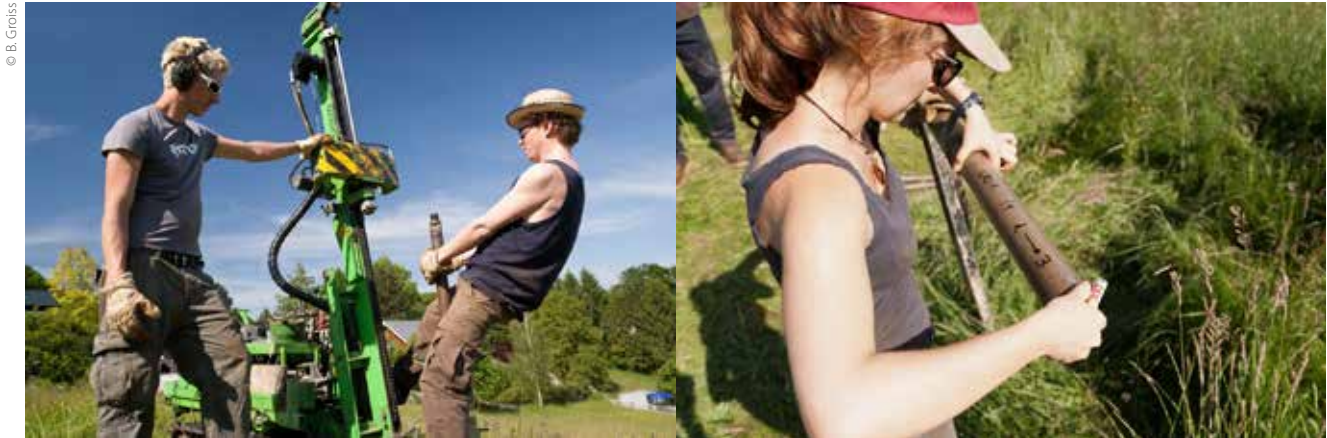
Field work in Gresten, Lower Austria: Two students use a drill crawler with pneumatic ram; a student marks the so-called inliner, containing the drill core.
